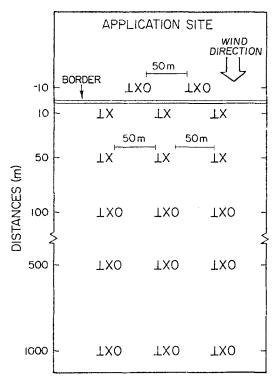
1 = AIR SAMPLING PUMPS AND RESIN FILTERS
